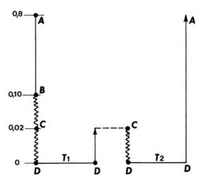
Fig.N°8- Feed scheme in case of plunge shaving
