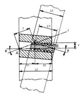
Fig.N°2- Indication for the calculation of stroke length in diagonal shaving
