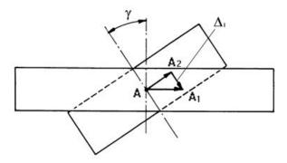
Fig.N°4- Indication for the vectorial calculation of effective cutting speed
