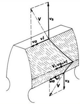
Fig.N°6- Speed vectors in the various point of the tooth
