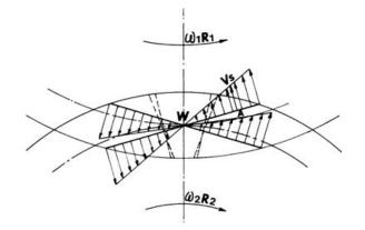
Fig.N°5- Indication for the calculation of cutting speed vector along the direction of tooth height
