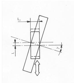
Fig.N°3- Indication for the stroke length in underpass shaving
