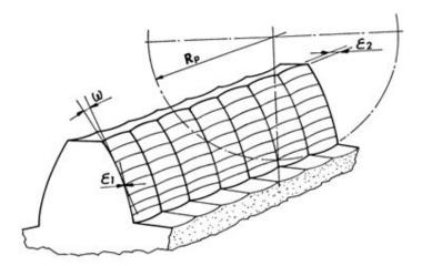
Fig.N° 1- Hobbing scallops along tooth flank
